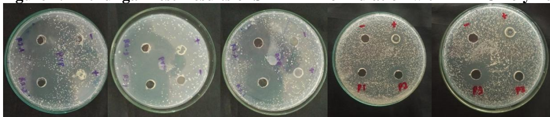
Figure 2. Antifungal Test Results of SMMDF Formulation with PVP Polymer
